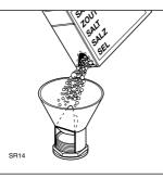
The salt container will require topping up periodically. You are reminded of this by the salt indicator light on the control panel which comes on when the salt has finished.
